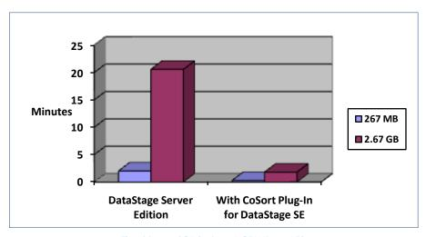
Fixed-key, ASCII Sort on 4-CPU IBM p650
