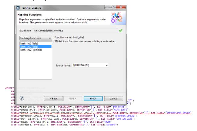
This is also known as a cryptographic hashing function. For any number of input bytes, the routine always returns a 32-byte hash code (in binary) that internally translates to a 44-byte, base64 value. Hashing is a useful technique for integrity checking. SHA-1, SHA-2, and SHA-2 OpenSSL are available.
